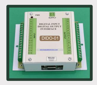
Digital Input & Output Module offers robust and versatile digital signal processing capabilities for industrial applications. With support for a wide voltage power supply range of DC 7 to 36V, it ensures compatibility with various power sources commonly found in industrial environments. It offers 15 Input CH for interfacing with external sensors. 15 output CH utilizes Darlington transistors, provides stronger driving capability with up to 500mA sinking current, built-in flyback diode protection
